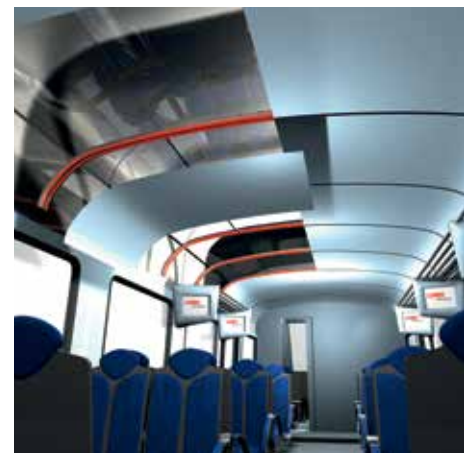
Ceiling Panel Bonding
