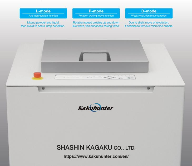
**Mixing force is increased by individual revolution and rotation control and step mode to eliminate lumps.** In mixing powder and resin, powders are easily formed into lumps and difficult to crush. The individual setup function for revolution and rotation speed can be used to prevent lumping for motion mixing and degassing.
