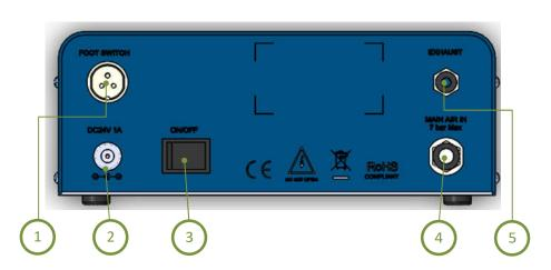
FIG. 3: External Controls - Back
